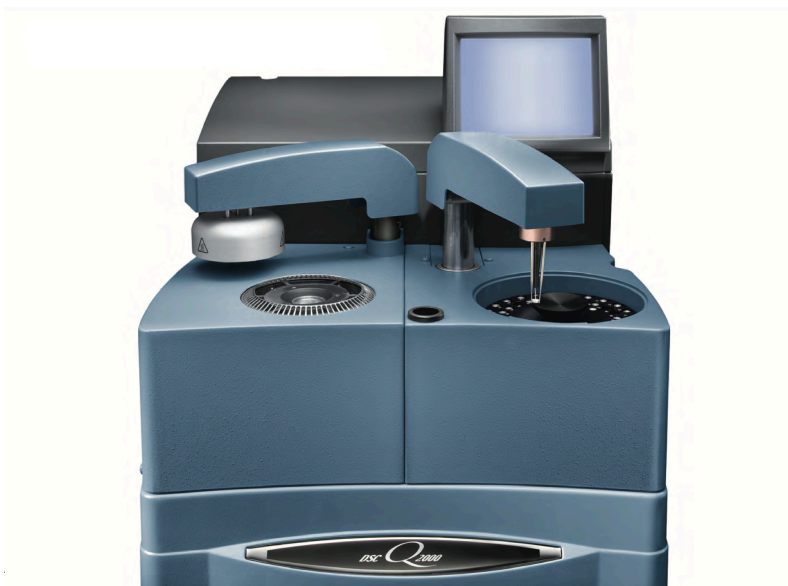
Figure 2.8 TA Instruments Q2000 DSC equipment (Adopted from [48] )
